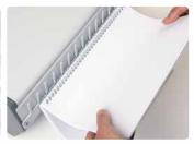
Pre-punched paper is loaded onto the integrated easy-loading wire holder.
