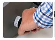
Fast and comfortable wire diameter changes adjusted by a simple hand wheel guarantee the perfect setup.
