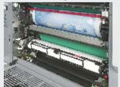
Automatic blanket cleaning device
