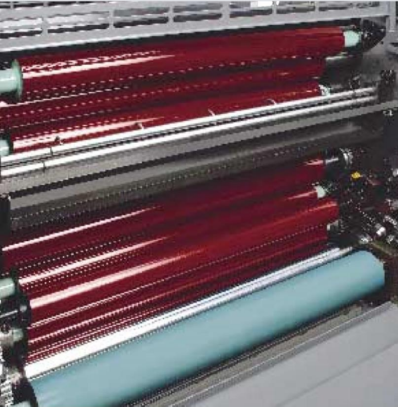
Inking and dampening mechanisms
