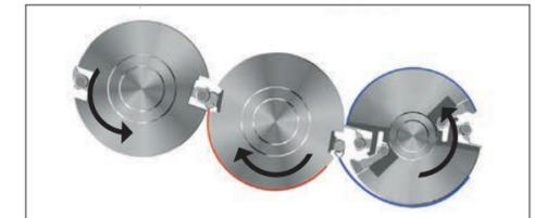
Three-cylinder sheet-reversing mechanism
