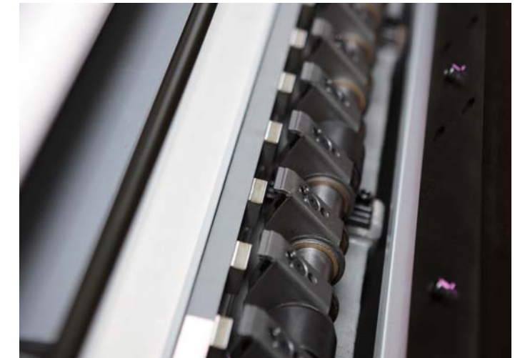
Double sprung gripper mechanism employing torsion bars
