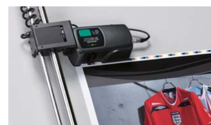
Printing density control system RYOBİ PDS-E SpectroJet
